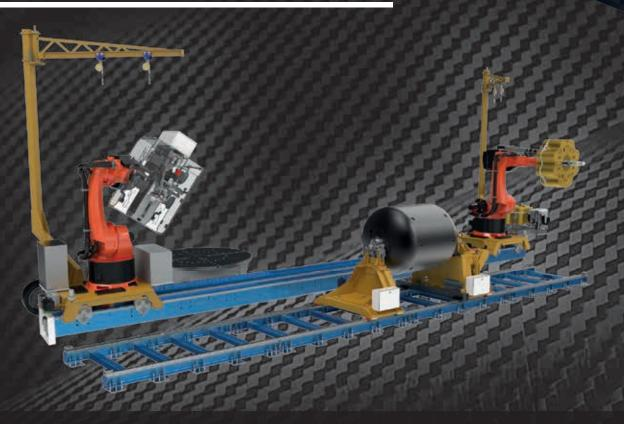
Innovative integrated AFP - FW - MILLING MACHINE for the production of cryogenic vessel in composite for aerospace application (type IV and type V).
